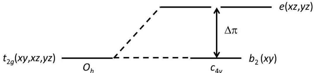
The  $d\pi$ -orbital splitting for a tetragonal nitrido-metal complex is shown above.
